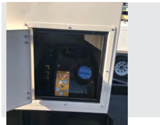
DEF Tank Location
